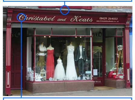
**Fascia** - provides an area to display details about the business run from the shop, saying what it is, when it was established, contact details etc. It can be angled forwards which aides details being read from the pavement.
