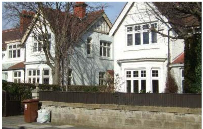
The third main wall material – a covering – is roughcast render, used on the majority of the early to mid-twentieth century buildings, many of which are built in the cottage revival style. Roughcast is used either on the entire building or on the first floor only, above a red brick ground floor. Rendered panels are also used with false half-timbering on several buildings. Some render
