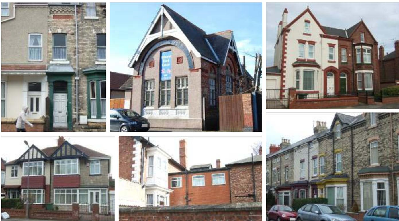
*Render (top left, top middle) and stone cladding (bottom left) damage appearance and can harm the fabric beneath, too, in the long run. Masonry paint (top right, bottom right) destroys the harmony of terraces or semis. Poor choice of brickwork and detailing (bottom middle) makes additions stand out unnecessarily.*
