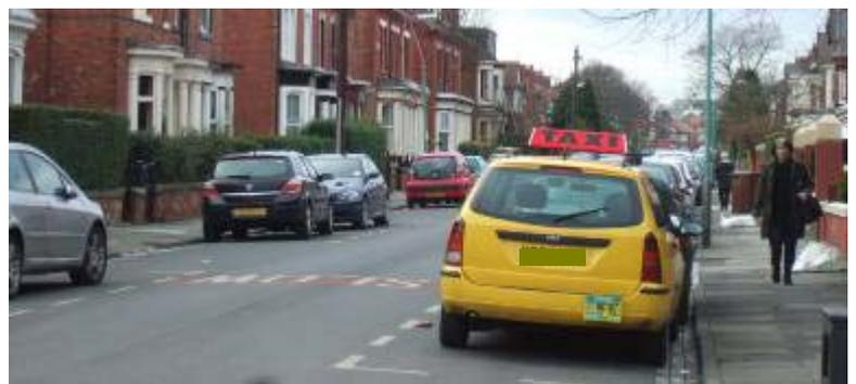
Most pavement are flagged, mostly concrete. The use of flags is important to the suburban character and more appropriate than tarmac which tends to spoil the scene where it is used (notably on parts of Hutton Avenue). Blue scoria blocks, a by-product of the iron industry, are an important locally distinctive material used frequently for gulleys and crossings. Scoria blocks should be
