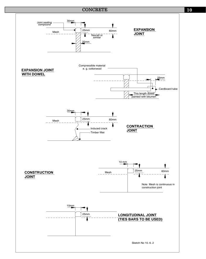
Sketch No 10.6.2 TYPICAL REINFORCED CONCRETE LAY-BY JOINTING DETAILS
