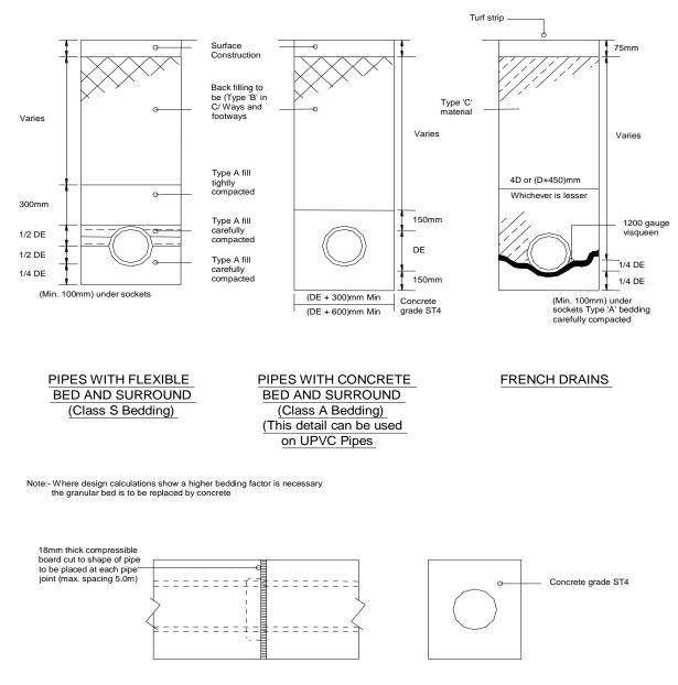
DETAIL OF FLEXIBLE JOINT IN CONCRETE BED AND SURROUND
