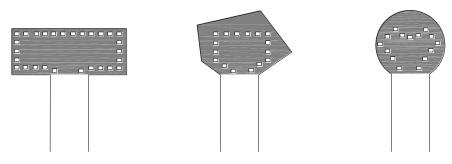
Different turning spaces and useable turning heads
