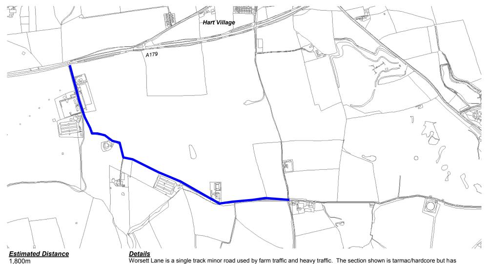
Worsett Lane is a single track minor road used by farm traffic and heavy traffic. The section shown is tarmac/hardcore but has seriously deteriorated due to weathering. The proposal would be to resurface the whole section with a sealed tarmac surface. There is no funding identified for this proposal at the present time.
