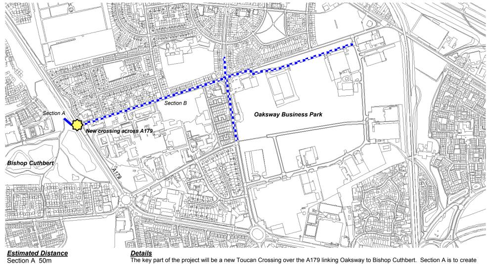
1,450m total The key part of the project will be a new Toucan Crossing over the A179 linking Oaksway to Bishop Cuthbert. Section A is to create connections to existing cycleway/walkways. Section B involves signposting, advanced stop lines and advisory road links on existing roads. This is a Local Growth Fund (LGF) supported scheme that was completed in May 2017
