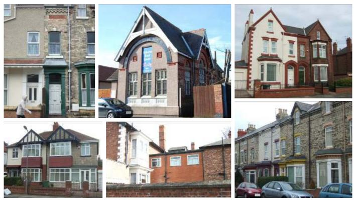
Render (top left, top middle) and stone cladding (bottom left) damage appearance and can harm the fabric beneath, too, in the long run. Masonry paint (top right, bottom right) destroys the harmony of terraces or semis. Poor choice of brickwork and detailing (bottom middle) makes additions stand out unnecessarily.
