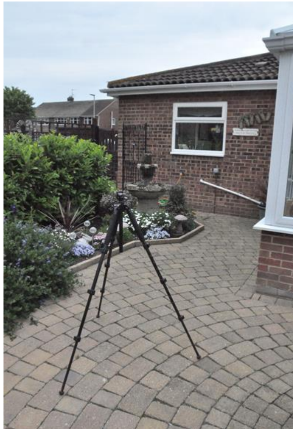
Figure 3: Microphone tripod positioned as was the applicant's microphone tripod, revealing the reflecting wall.
