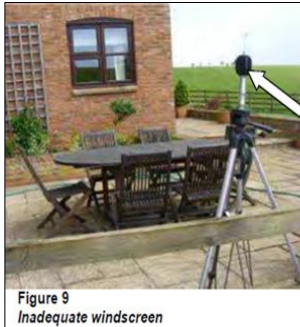
Figure 5: The DMK wind shield, an “inadequate windscreen” according to SGN1 of the IOAGPG
