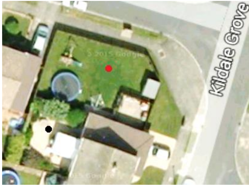
Figure 4: Red spot shows appropriate microphone position available to applicant; black spot shows position chosen by applicant.
