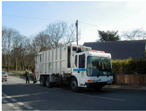
Figure 3.7 Compaction Refuse Collection Vehicle in the Tees Valley
