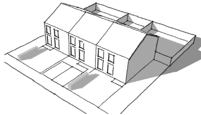
Figure 58: Terraced parking (short runs)
