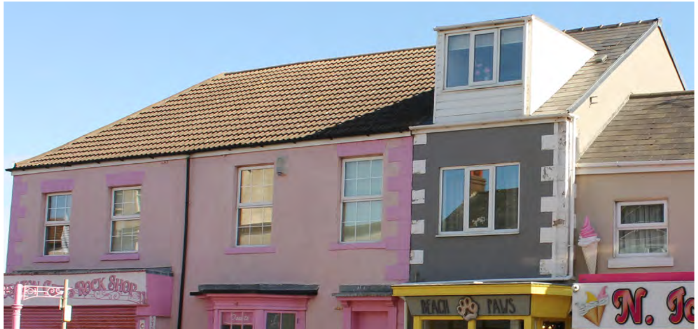
Modern concrete tiles are not an acceptable material on historic buildings in the conservation area. The loss of chimneys also presents a featureless roofscape
